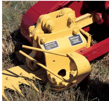
Straight-line motion of the drive head provides fast, smooth cutting combined with less wear on the knife assembly and hold-down clips.
