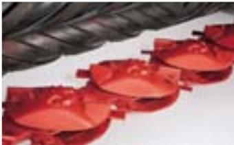
Two heavy-duty knives on each disc spin at 3,000 rpm for fast cutting without plugging.
