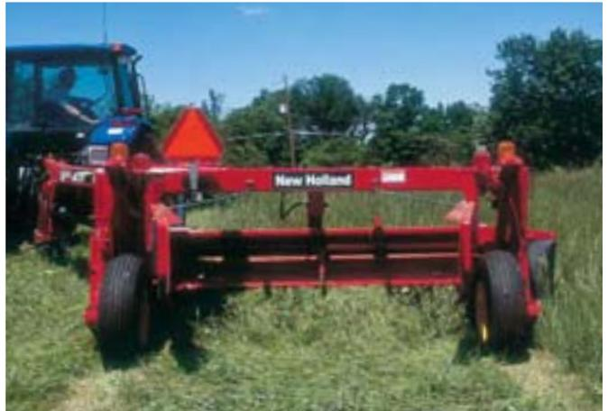
*A center-pivot, swivel-hitch tongue provides even better maneuverability and tight corner cutting than a standard drawbar center-pivot.*
