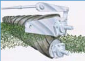
crimp and crack stems evenly along the entire length of the plant, so you get fast drydown yet retain protein-rich leaves. Adjusting roll pressure is easy. No tools are required. Critical roll gap adjustment is made with one adjusting bolt per side, no removing or adding shims.
