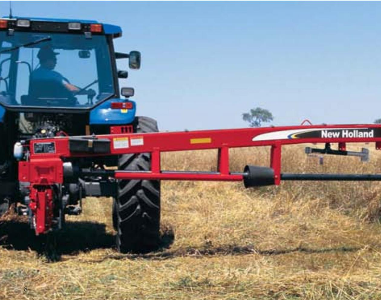
tongue design you can enjoy swivel hitch-like convenience and performance without the need for a three-point hitch or drawbar extension. You can mow at most any angle and make square and over-square corners without vibration or noise.
