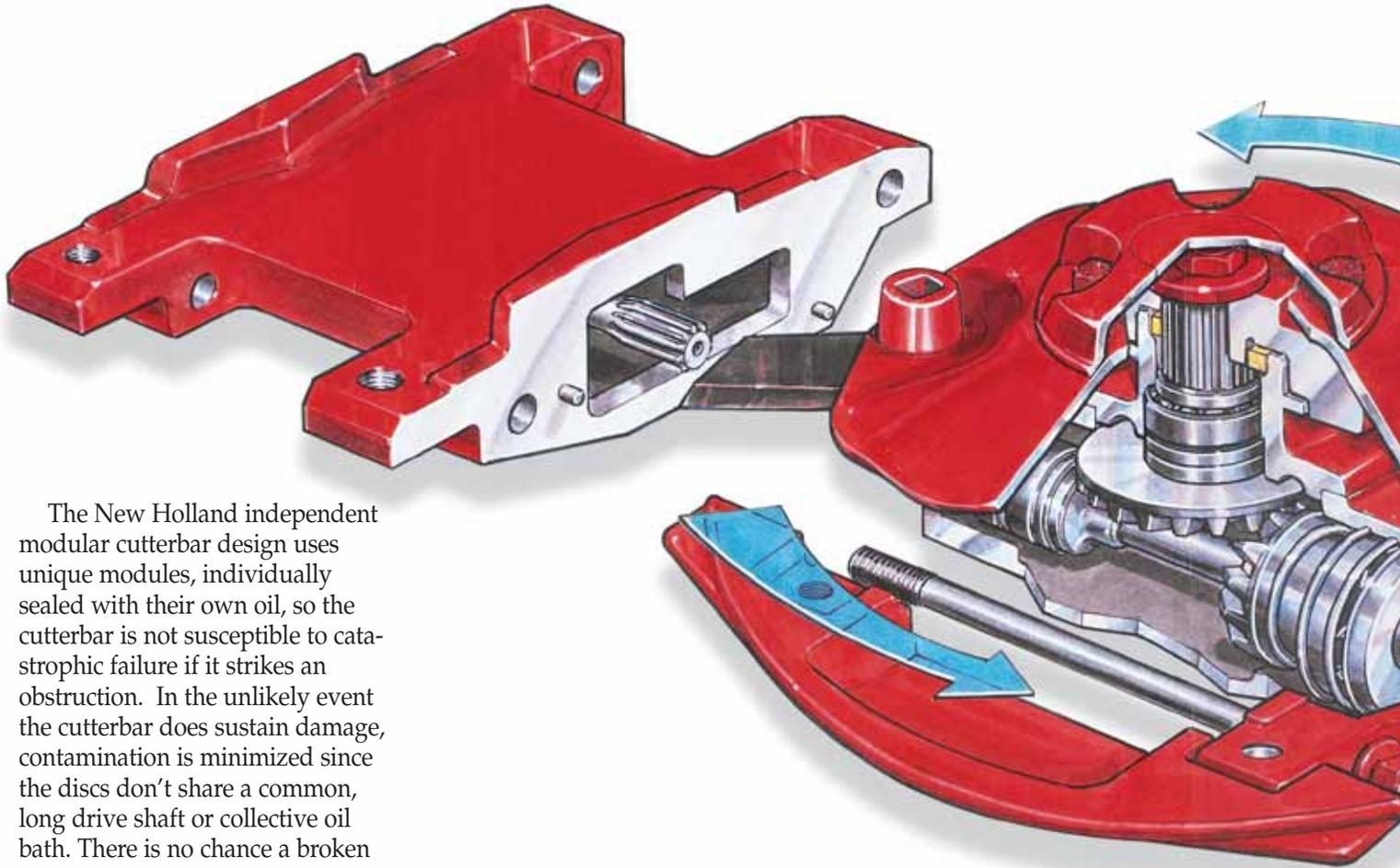
The New Holland independent modular cutterbar design uses unique modules, individually sealed with their own oil, so the cutterbar is not susceptible to catastrophic failure if it strikes an obstruction. In the unlikely event the cutterbar does sustain damage, contamination is minimized since the discs don't share a common, long drive shaft or collective oil bath. There is no chance a broken gear tooth could migrate into other components and cause major damage.
