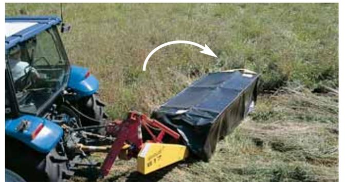
*A spring-loaded breakaway latch protects the cutterbar by allowing it to swing back the instant an object blocks the cutter path. Simply back up to re-engage the latch.*
