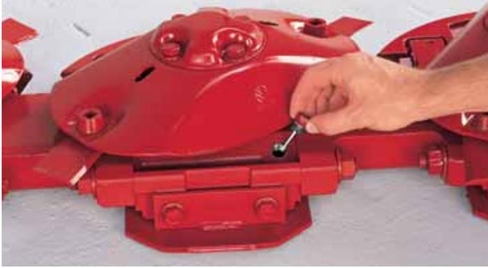
*Cutter bar service couldn't get much easier. Check the oil in the modules every 50 hours with the convenient dipstick provided in the cap. Change the oil once a season or every 200 hours. For even more convenience, only one type of oil (80W90, GL5) is needed for all locations.*
