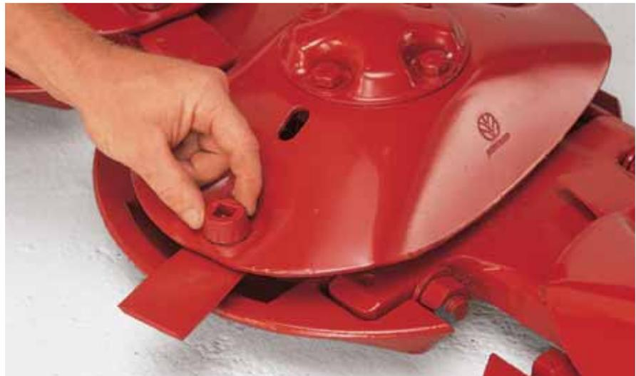
*Smooth profile discs are  $\frac{3}{16}$ " thick and heat-treated for strength and impact resistance.*
