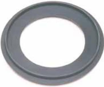
*Unique "T-seal" washer is positioned between each pivot arm and bevel gearbox to prevent sand and dirt from entering and damaging the pivot bushings. An additional lip seal is positioned toward the outside of the pivot arms to protect against damage from debris.*
