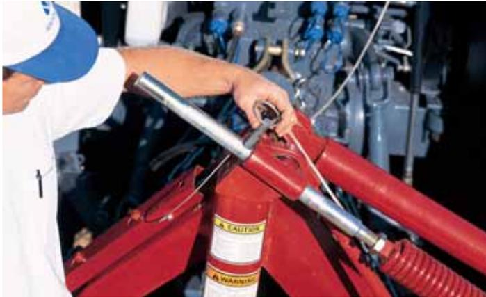
*Convenient jack stand storage and installation. Remove the tethered pin to install the jack. Flotation spring force is released automatically.*
