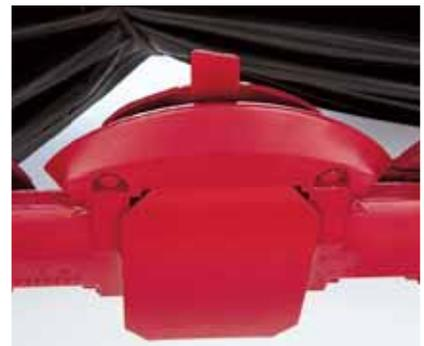
*Skid shoes are  $\frac{1}{4}$ " thick and 8" wide to protect the disc modules from obstacles. They extend behind the module several inches for optimum flotation and extended wear life of the shoe. Their unique shape works with cutterbar tilt to provide a broad range of cutting heights.*
