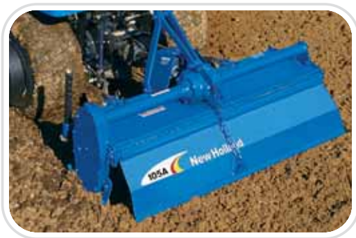
Rotary tiller uses curved steel tines to prepare seedbeds or control weeds between the rows.
