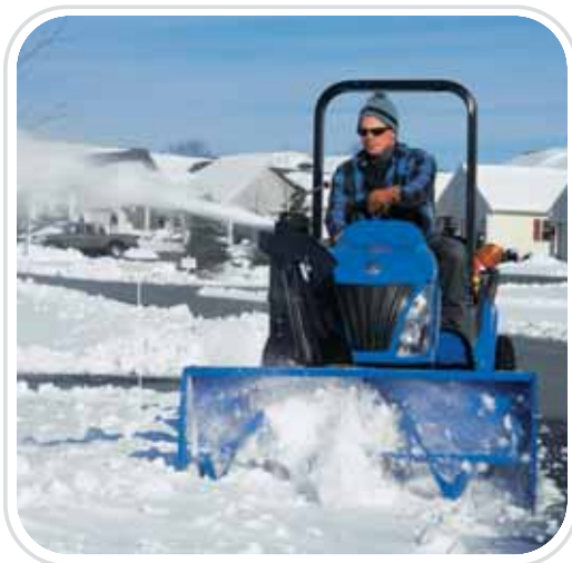
Front Quick-Attach snow blower cuts through snow up to 20 inches high, using a two-stage process to turn your Boomer into a powerful snow removal machine.
