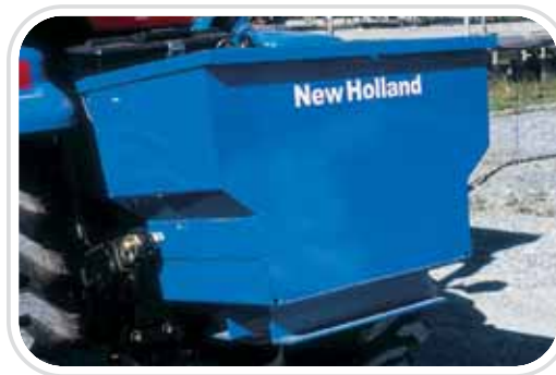
Ballast box helps provide the counterweight necessary when working with some heavy, front-mounted implements.
