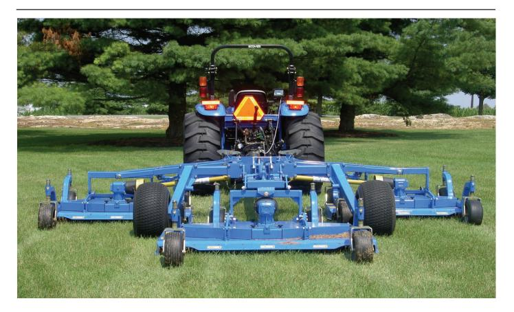
The New Rear Discharge Flex-Wing Finishing Mower series has been designed for golf courses, parks, or large areas. Each model features 3 floating decks with 4 wheels on each deck.
