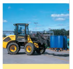
Precise, parallel forklift path eliminates the need for manual correction so operators can focus on load placement rather than load leveling.
