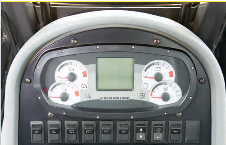
The instrument cluster provides system information with analog gauges and warning lights.
