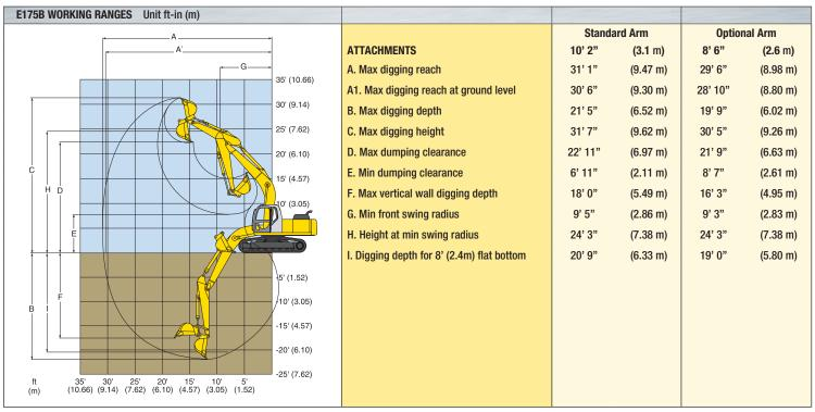
Measurements shown are for machines equipped with the 0.82 cu. yd. (0.63 m<sup>3</sup>) bucket.
