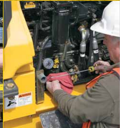
The swing-up hood allows easy access to site windows and fluid dipsticks and filters.
