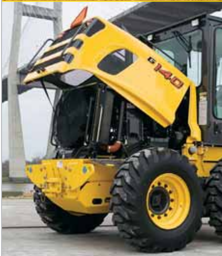
The fiberglass hood swings open assisted by charged cylinder supports. This provides easy access for routine engine maintenance.
