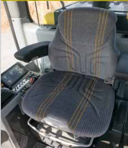
Adjustable suspension seat, arm rests and steering wheel allows each operator to achieve a comfortable position.
