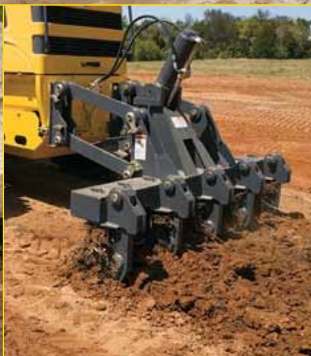
The optional parallelogram ripper provides over 17" of ground penetration, even in hard-packed soils.
