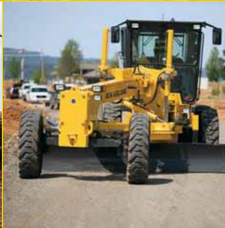
25 degrees of articulation angle (left and right) maximizes maneuverability, visibility and control
