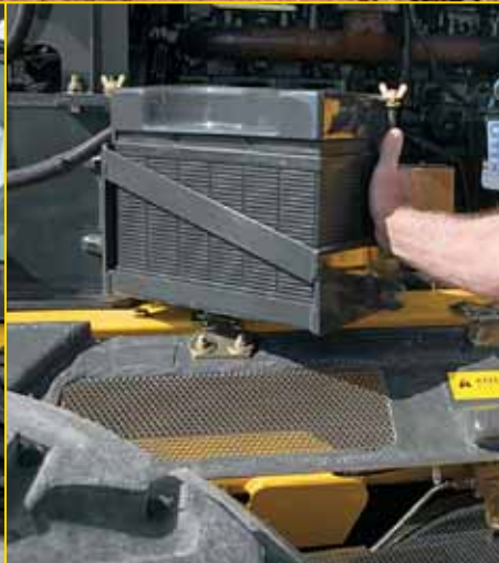
Two swing-out 1010 CCA maintenance-free batteries, one conveniently located on each side of the engine compartment.
