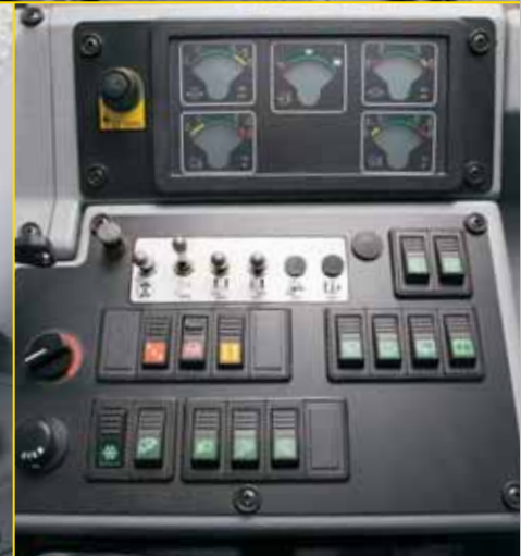
Easy-to-read gauges allow monitoring of fluid levels and operating temperatures.
