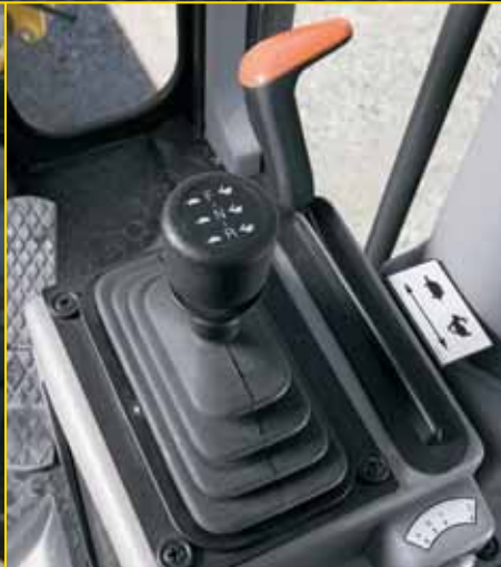
F-N-R bump shifter with eight forward speeds and four reverse speeds.
