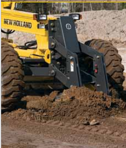
The front scarifier offers 20.75 inches of lift for excellent ground clearance and 12.5 inches of ground penetration.
