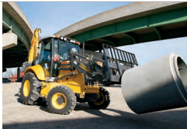
Model B95B TC (Tool Carrier) delivers true self-leveling both up and down, making it perfect for use with forks. The B95B TC has an optional hydraulic quick coupler so you can easily change attachments.
