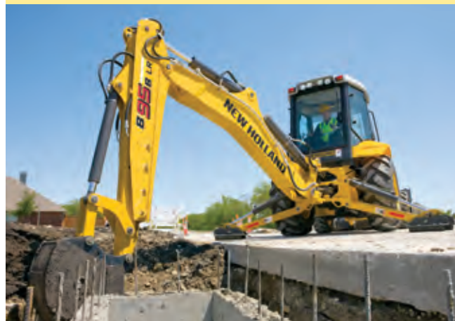
Model B95B LR (Long Reach) combines the B95B base unit with the longer stick of the B110B loader backhoe – making it a 15-foot machine. It's ideal if you're looking for added reach with better fuel consumption than larger machines.
