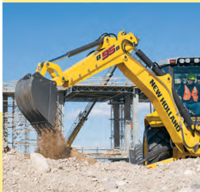
Model B95B LR (Long Reach) combines the B95B base unit with the longer stick of the B110B loader backhoe – making it a 15-foot machine. It's ideal if you're looking for added reach with better fuel consumption than larger machines.
