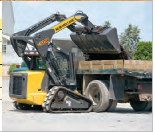
\*Base unit plus full fuel tank, 165 lbs (75 kg) operator, 72" dirt and foundry bucket, and 12.6" (320 mm) track belt width
