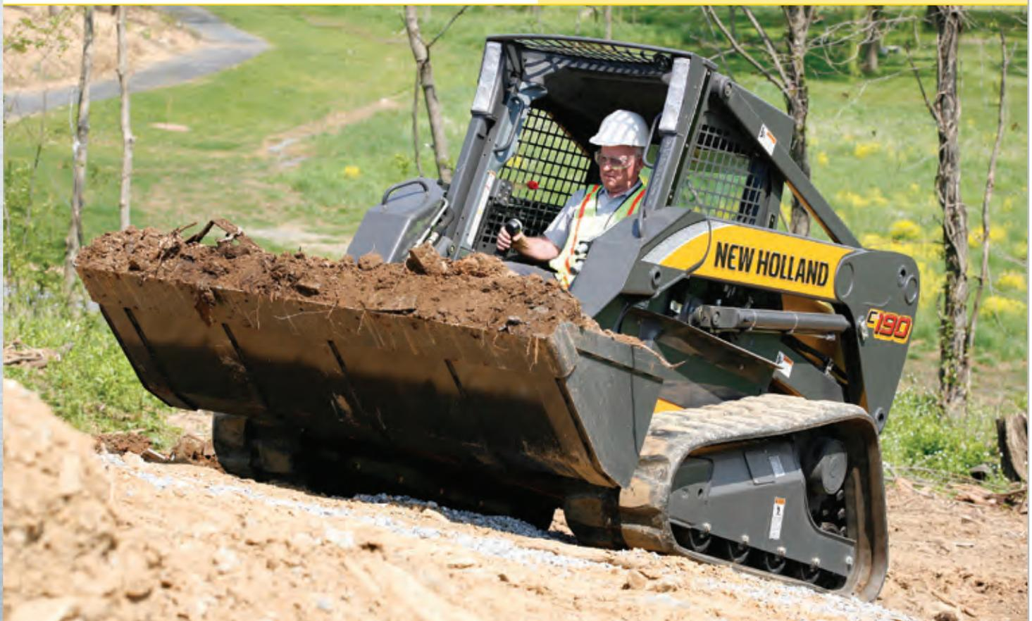
With Super Boom® vertical lift linkage, the higher you lift the load, the farther forward you reach, achieving outstanding dump height and reach.
