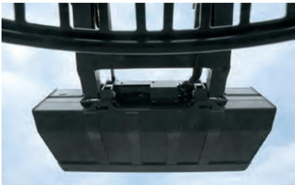
The see-through area on the cab roof provides a clear view to the bucket, even when it is positioned at full height.
