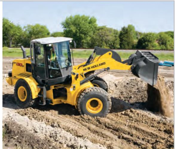
Standard limited slip axles deliver greater traction while the long wheelbase and short turn radius allow for extra-smooth maneuvering.
