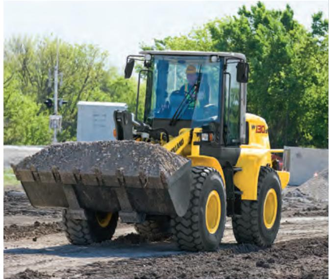
Flat glass provides an unobstructed view to the bucket and the worksite.
