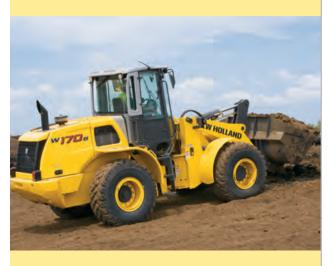
Standard limited slip axles deliver greater traction while the long wheelbase and short turn radius allow for extra-smooth maneuvering.
