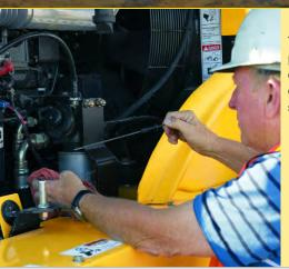
You can reach all daily check points from ground level, and can easily reach major engine components through lockable, swing-open service doors.
