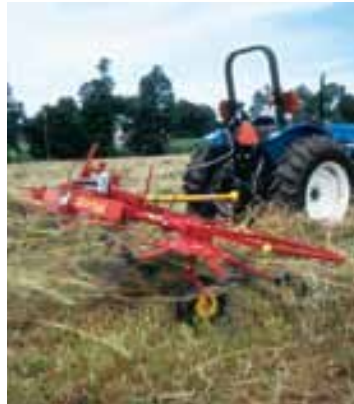
The Model 163 tedder features four rotors to cover an expanded 16'5" width, yet folds to a width of 9'6" to maneuver easily through gates or narrow roadways.
