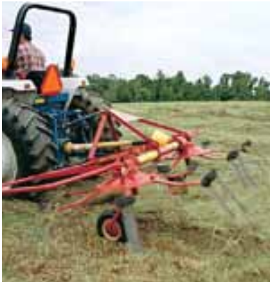
The mounted Model 157 tedder fluffs a 8'6" swath and maneuvers easily around smaller fields. The left-hand rotor tine bar flips up for narrow 8' transport.
