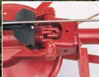
Digidrive couplings on New Holland tedders are virtually maintenance free. Workloads are spread evenly over 12 intermeshing forged and heat-treated fingers. The couplings offer high resistance to wear and eliminate open universal joints.
