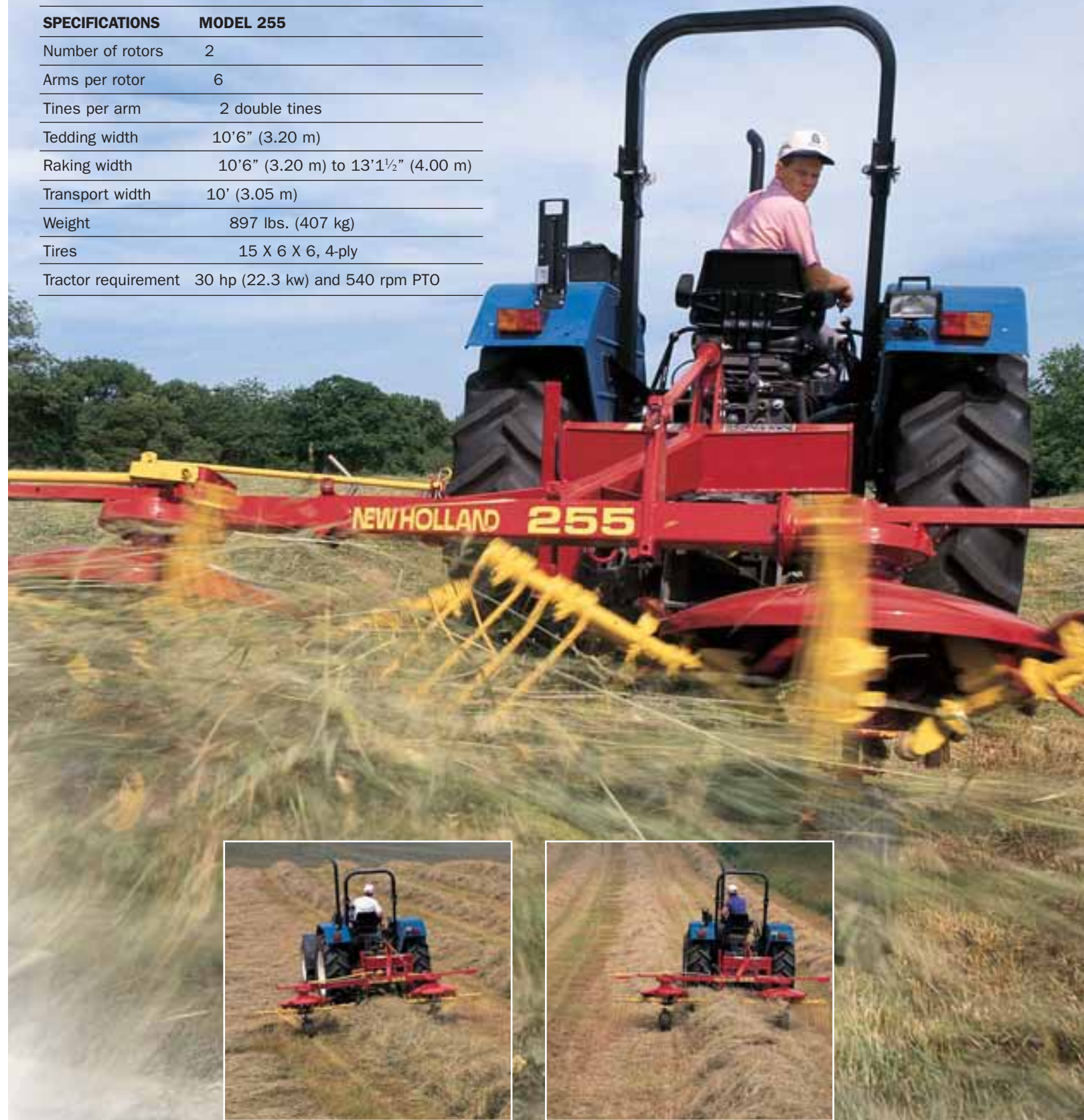
Rake swaths up to 13 feet wide into windrows ready for baling or chopping.
