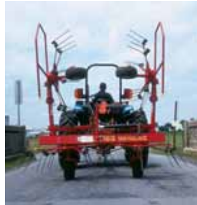
The Model 163 tedder features four rotors to cover an expanded 16'5" width, yet folds to a width of 9'6" to maneuver easily through gates or narrow roadways.
