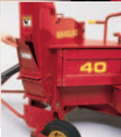
*A convenient access door makes it easy to check fan-blade-to-band clearance and to replace fan paddles.*
