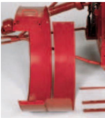
*Replaceable fan wrapper liners are made of abrasive-resistant steel to increase blower life.*
