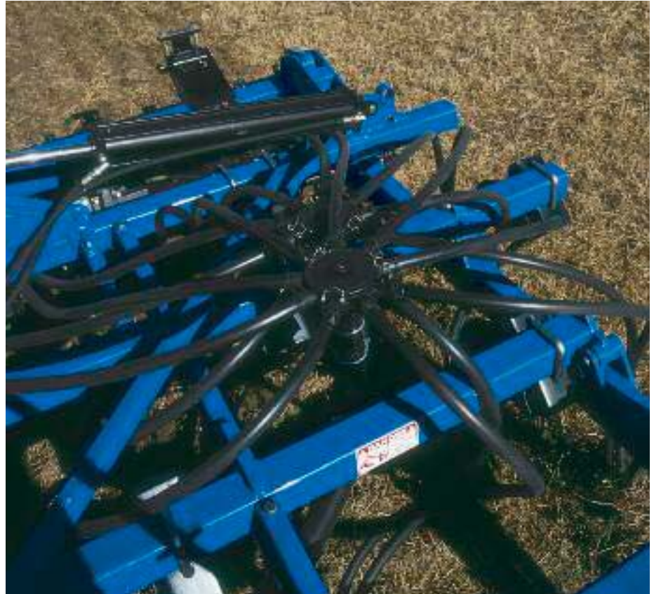
Easy Flow headers provide unbeatable product flow and gentle seed handling from primary to secondary lines. The design makes for easy clean-out access and service.
