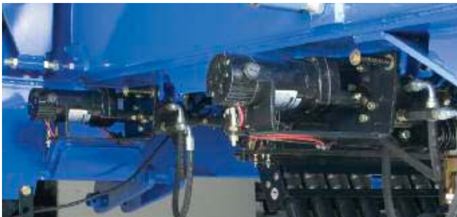
Variable rate metering uses an independent drive for each meter for precise metering even at low roller speed. This allows you to electronically control product rates on-the-go from the cab. It also allows you to utilize field mapping and fully integrate your seeding and fertilization into your precision agriculture activities.
