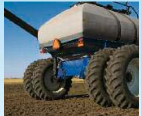
Dual grip tires for extra floatation in soft soils.
