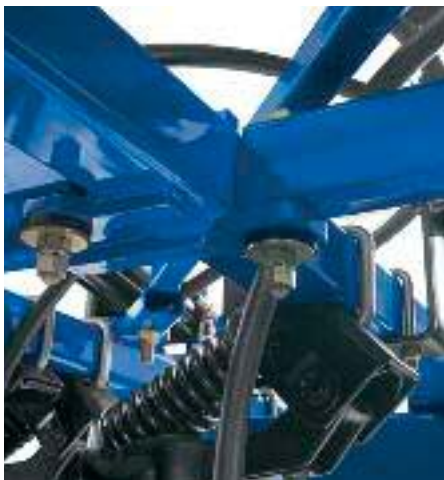
Self-lubricating bushings, chrome pins and durable polyurethane pads are located at frame flex joints for long frame life and continued depth accuracy.
