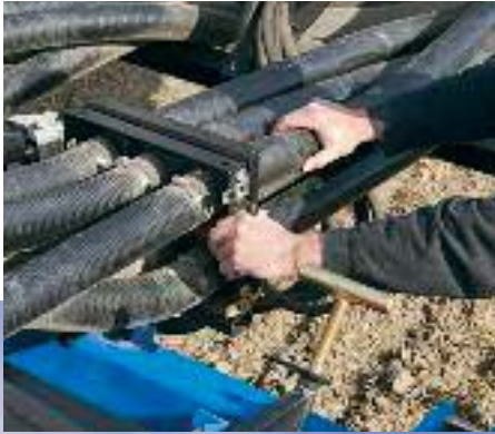
Quick-Connects let you hook up to seeding or banding tools quickly and easily—especially helpful if you use your air cart on different tools.
