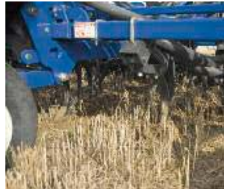
The floating hitch gives improved front-to-back land following.
