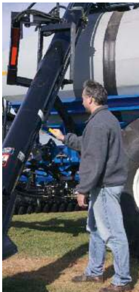
You can fill and empty tanks fast with large, orbital-drive augers.
