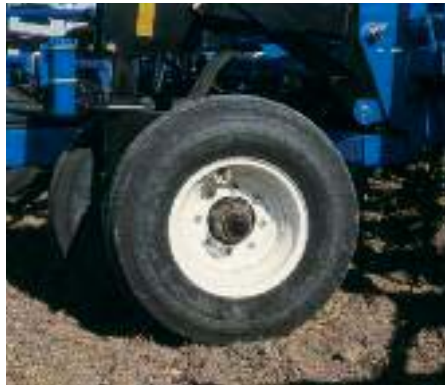
Dual walking casters provide optimum flotation.
