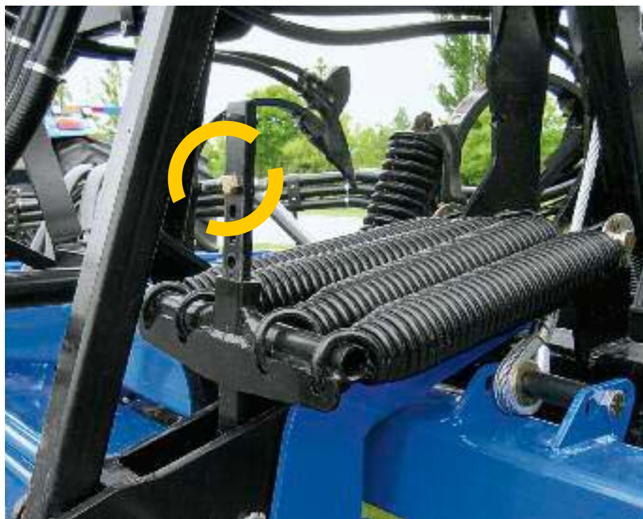
This patented variable packing pressure system allows you to tailor pressure quickly, as needed.
