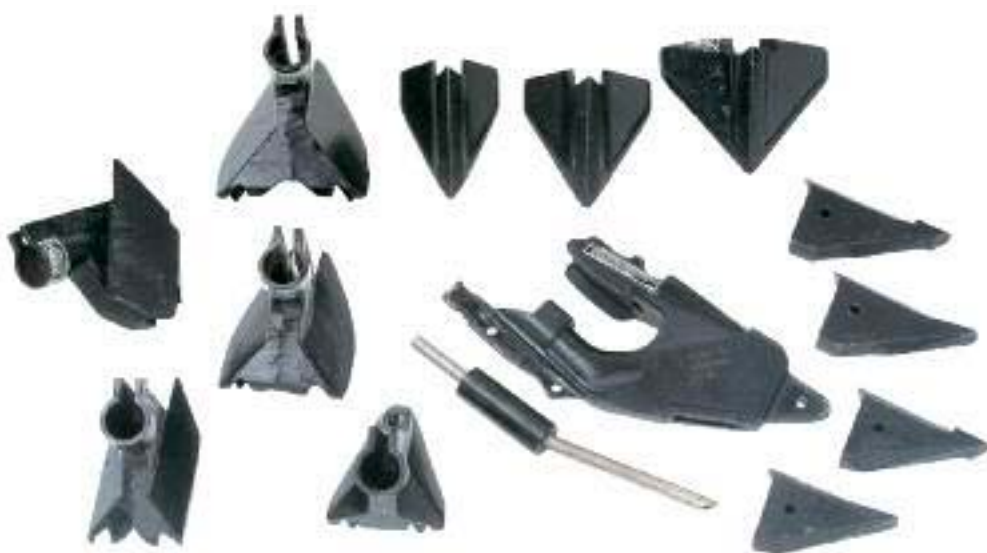
The main Stealth™ opener body mounts on the shank. A replaceable tip is secured to the main body with a roll pin. Double-shoot attachments bolt on to the rear of the main body.
