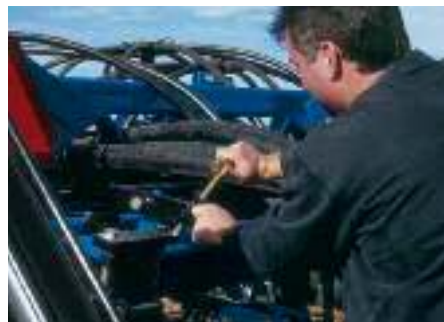
You set the depth for the entire machine at a single point.
