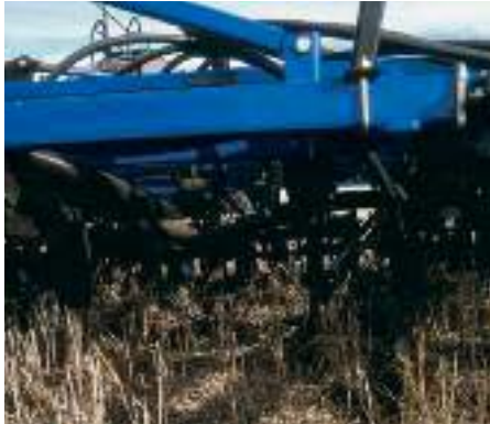
32 inch frame clearance lets residue flow through the drill.
