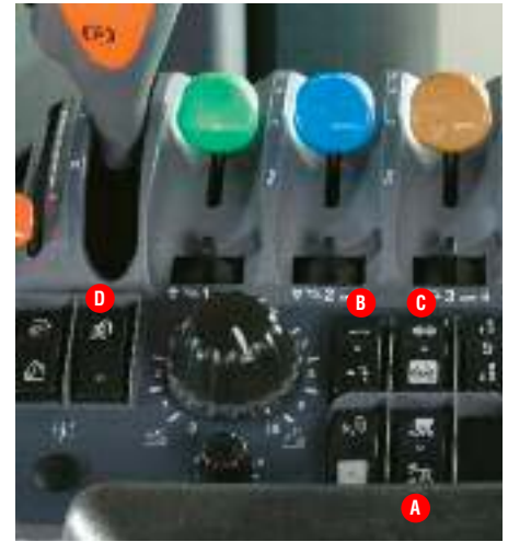
Switches are conveniently located on the right-hand armrest control console for A) Auto Shift, B) Front-wheel drive engagement, C) Automatic Diff Lock and D) Custom Headland Management.
