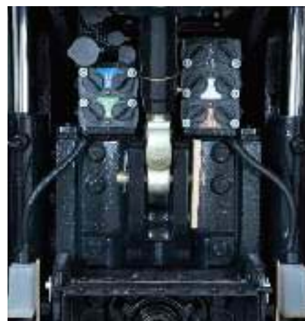
The in-cab hydraulic remote levers are color-coded to match the quick couplers so you can easily keep track of hydraulic operations.
