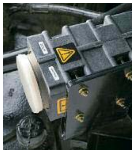
Add the optional ground speed radar sensor to the performance monitor and you can track precise ground speed and wheel slip, important factors during spraying, planting and tillage.
