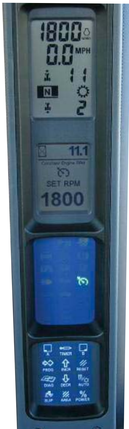
Simply use this keypad to change the information displayed on the digital readout for the Performance Instrumentation.
