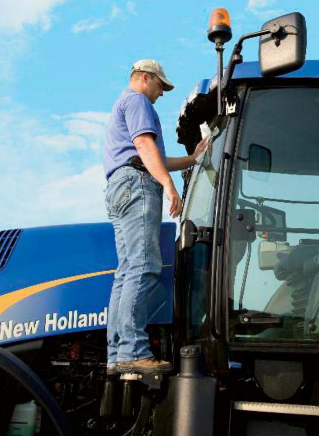
The standard front window step makes it easy to clean windows and reach the front wiper, front cab roof lights or top of the cab to install a GPS guidance receiver.
