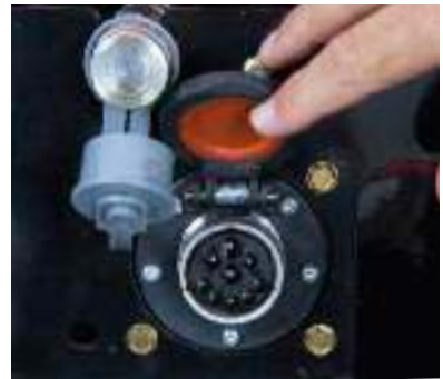
Hydraulic Trailer brake option and plug to control ISO 11783 implements of any brand
