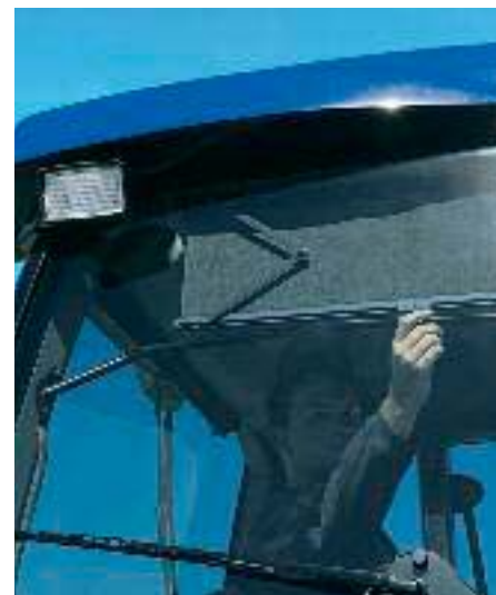
Add the windshield wiper and sunshade options for the right-hand window for clear views no matter what the weather. Wiper/washers for the front and back, and a front sunshade are standard.
