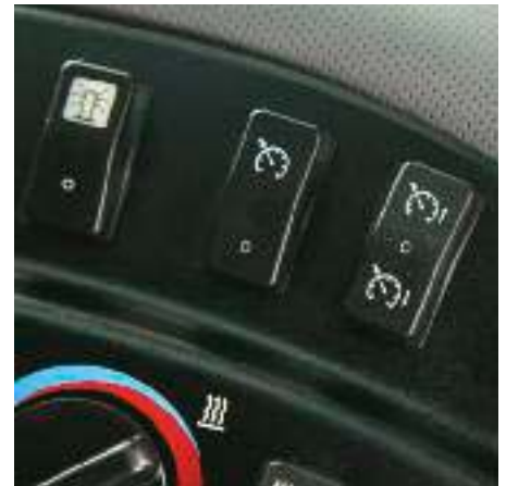
Constant Engine Speed “cruise control” switches to your right allow you to maintain a constant speed and save fuel. It’s one of the perks that comes with full-authority electronic engine management.
