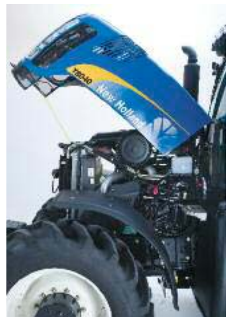
For complete engine access, the one-piece hood tilts up. No tools needed and no extra panels to remove.
