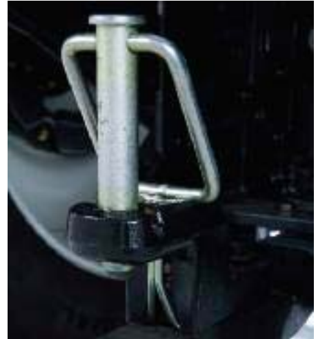
A swinging drawbar is standard equipment, and a high-capacity, heavy-duty drawbar is optional for applications where extra-heavy upward and downward loads are expected, such as with front fold planters, liquid manure wagons and large grain carts. The auto-pin hammerstrap (shown above) automatically drops and latches the pin when you hook up to implements.
