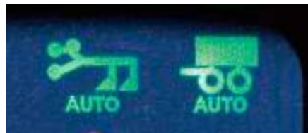
The Auto Shift icons appear on the instrument panel when the Auto Shift switch is depressed.
