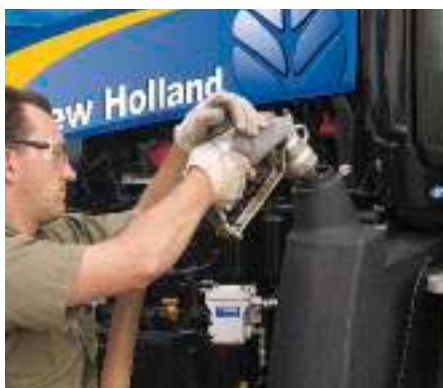
The fuel tank fill point is right beside the steps where it can be filled easily from ground level.
