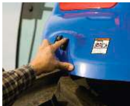
Fender switches for the three-point hitch and hydraulic top link provide convenient control from the ground.
