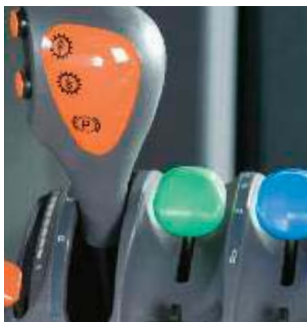
The in-cab hydraulic remote levers are color-coded to match the quick couplers so you can easily keep track of hydraulic operations.
